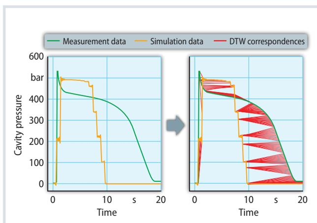
**Fig. 2.** Measured and simulated profile of the cavity pressure and computation of the DTW correspondences [27] Source: IfW and VM; graphic © Hanser
