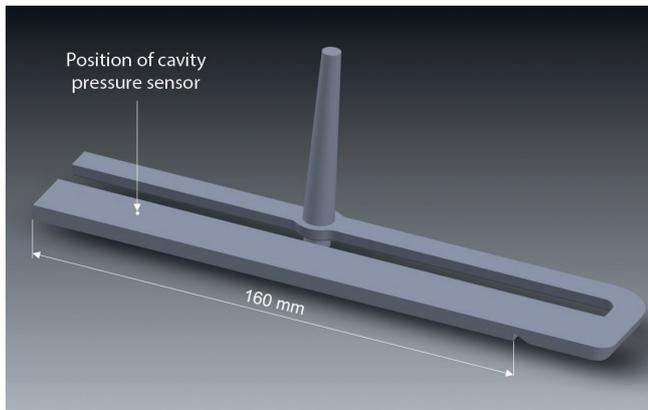
**Fig. 1.** This flat bar was used for determining the real and simulated part properties © IfW
