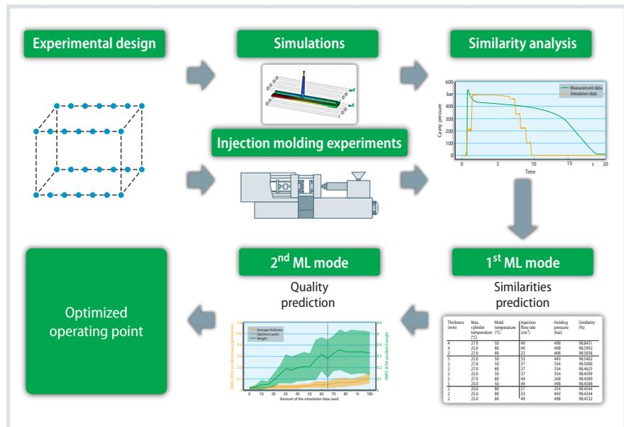
Fig. 3. Concept of the ML models for data-driven determination of the optimum operating point Source: IFW; graphic: © Hanser
