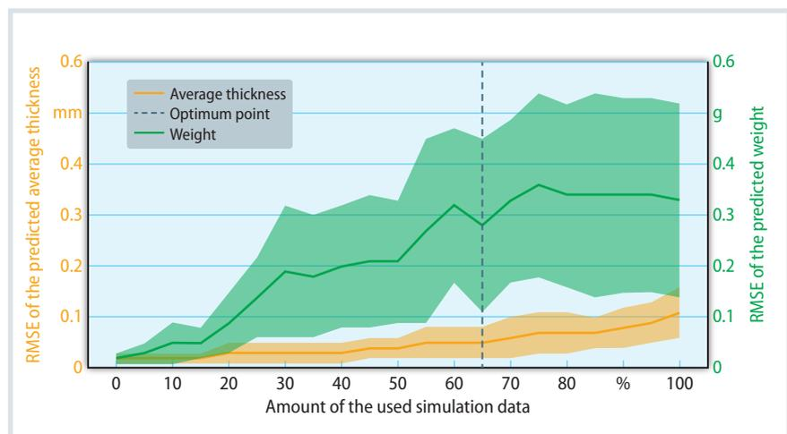
Fig. 4. Results for prediction of the part thickness and weight, shown in dependence on the proportion of the used simulation [27]; RMSE: root mean square error Source: VM; graphic: © Hanser
